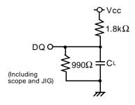
Fig.1 Output load
